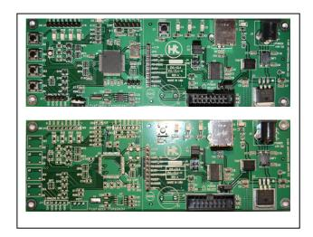
EVL-CL4 (Without Host Controller) and EVL-CL4-H (With Host Controller) are development boards for Haidar's Embedded Display Modules. They are used to quickly evaluate and demonstrate the functionality of display module.
