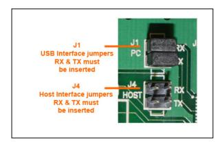
When both RX and TX of jumper J1 are installed, the board is connected to the USB. When both RX and TX of jumper J4 are installed, the board is connected to the Host controller via J5. One jumper J1 or J4 must be installed at a time.
