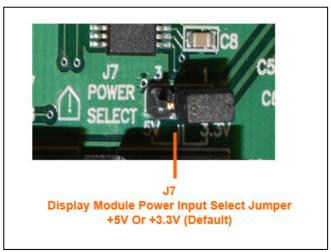
Warning: be sure that the power to the display module is within the operating range of the module. Exceeding the power to the display module over the typical ratings will damage the display module.
