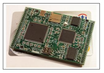
It is a fast, simple and inexpensive production solution for adding a Graphical User Interface to an embedded system. SegeNT GUI Controller Board contains everything needed to drive the user interface. It just needs to be attached to a simple display interface board and the human interface is ready for production.
