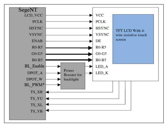
For 24-bit RGB displays, SegeNT R5 will be connected to the Display R7 and the same for the other colors. The display R1, R0, G1, G0, B1 and B0 must be connected to ground.
